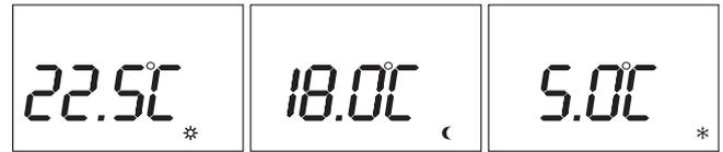
Press the +/- button to change the temperature of each mode then press **OK** to confirm and go to the next **MODE** and exit to the temperature setting screen by pressing **CONFIG**.
