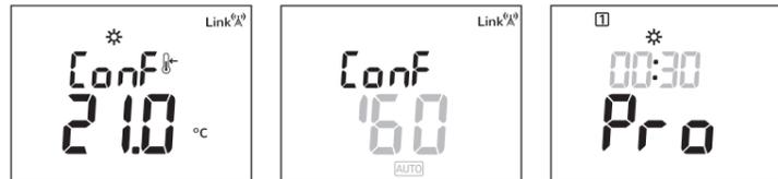
minutes. Finally, set the start and end time for each temperature setting **☼** (Comfort) **☾** (Eco) during the week.
