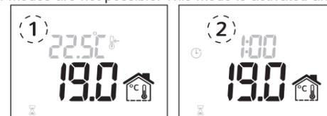
**RUNBACK/SETBACK:** RunBack mode is designed for when the thermostat is installed in areas where restricted user control is required such as rental or holiday accommodation, limiting the temperature and time the appliance is switched on.
